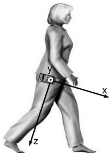
Fig. 2: Mounting position of cell phone and coordinate system of the accelerometer.
